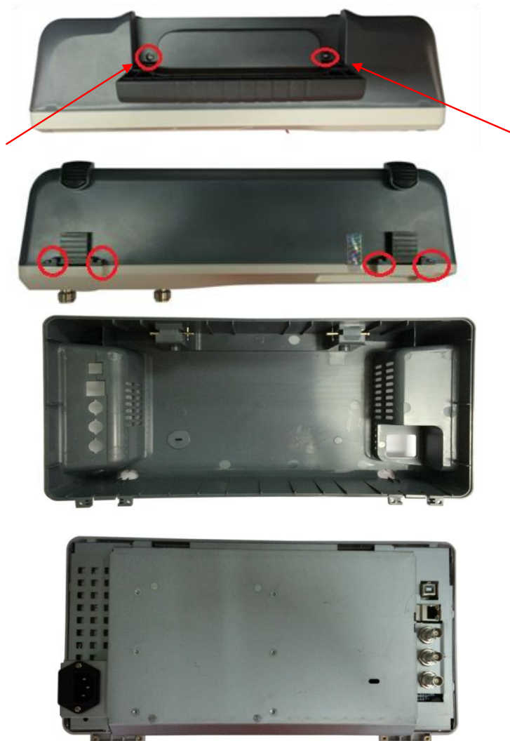
Figure 4-1 Removing the Rear Panel Screws
